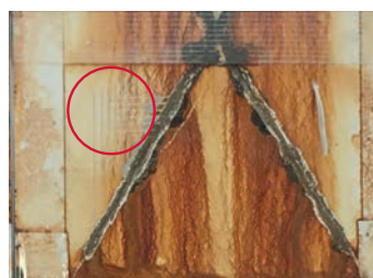
Salt spray test result of a 2K epoxy white coating after 1000 hrs treatment
